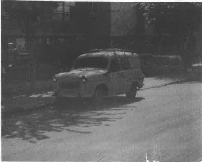
The first version of the Israeli built glass-fibre car, note its similarity to a Reliant.
