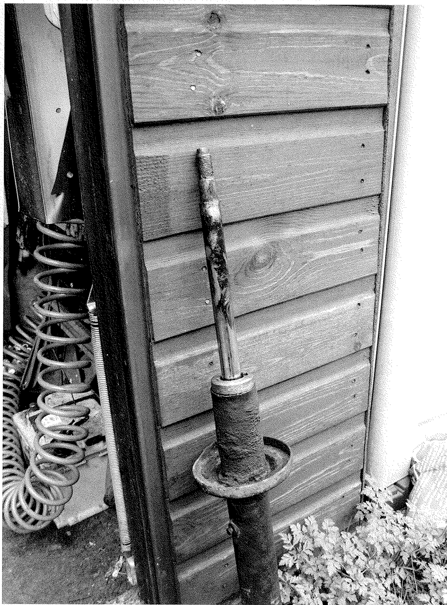
The strut after removal and after the spring had been removed for clarity, showing the gland nut fully clear of the strut body.
