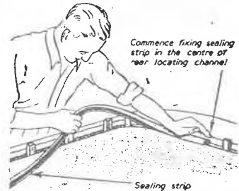
Fig. 4.—The fixing of the sealing strip is shown here.
