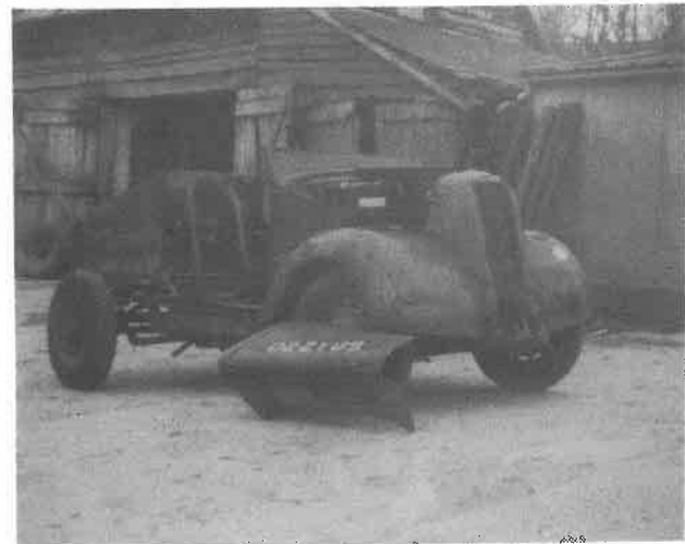
Photo shows an Allan Taylor Tractor (ex Army) based on a 7Y 8 h.p. Standard early engine. Rear axle has a reduction via chain wooden tipper body fitted. Ray Smith of Devises.
