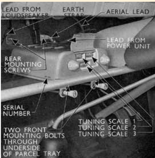
Photo 4. The receiver CR.152 / F for Standard models showing the flip-up cover over the display face.
