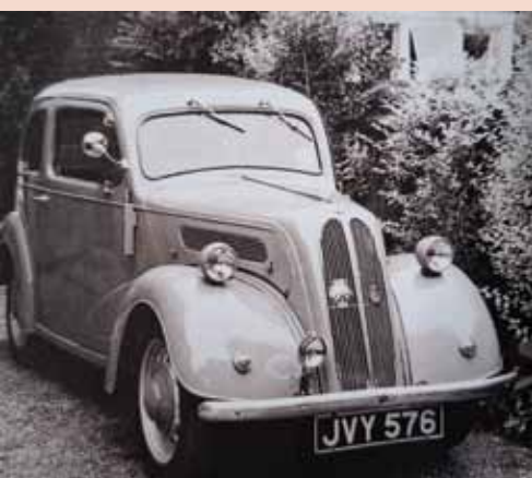
A 1954 Popular. This example has been enhanced by the presence of two windscreen wipers, semaphore and flashing indicators, as well as a driver's wing mirror.
