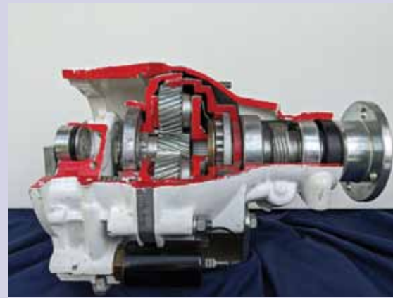
Photo 5. I have not found a photo of a Laycock 100E overdrive but this is the standard issue and it is thought that the 100E would be similar. It uses friction clutches to engage the overdrive.
