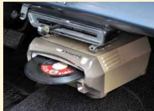
Photo 2. A Phillips version for 45 r.p.m. records and strictly singles, in all senses. The mounting arrangements do not compare with Ford's standards!
