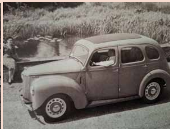
The revised Prefect for the 1949 season, with a new radiator grille and integral headlamps. The left hand steering is a recognition that Ford had begun to export its products to America.
